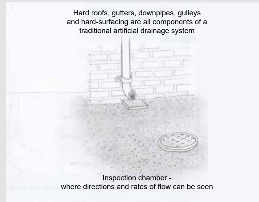
Examples of Visible Surface Components of a Traditional Artificial Drainage System
